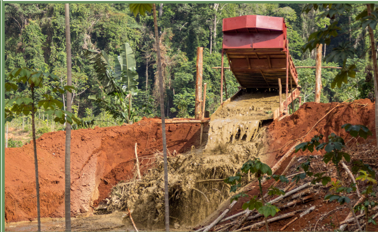
Marudi Mine, South Rupununi, Guyana. Sluicer pumping untreated water into an abandoned mine pit.
